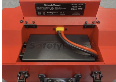
Figure 5 — The underside of the Safe-T-Mover with the battery in the battery compartment
