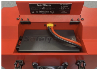
Figure 13 — The underside of the Safe-T-Mover with the battery in the battery compartment
