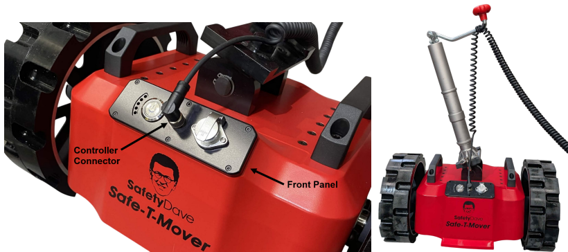
Figure 7 — A controller connected to the controller port on the front panel and wrapped around cable retainer
